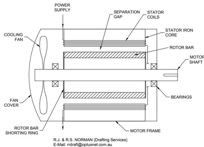
Figure 1. A simple cage induction electric motor design.
