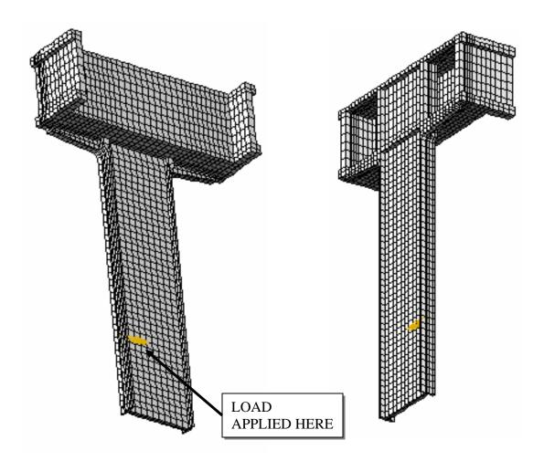
A HALF MODEL IS USED DUE TO THE SYMMETRY OF THE LOADING AND THE GEOMETRY. THE APPLIED LOAD IS 2475 POUNDS, WHICH IS EQUIVALENT TO 4950 POUNDS ON THE ENTIRE POST.
