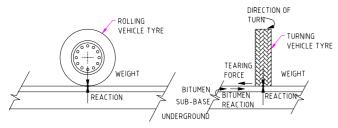
The drawing above shows a typical cross-section through a road and highlights the forces produced by a wheel contacting the surface.
