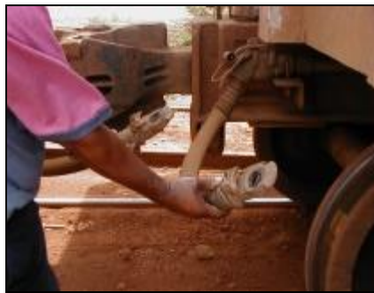
Figure A.2.3 Uncoupling Railcars
