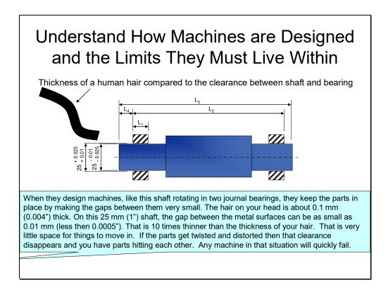
In the sketch the bearing diameter ranges 25.01 to 25.025 mm. Shaft diameter ranges 24.975 to 24.99 mm. Bearing to Shaft <u>diametric</u> clearance ranges from a possible low of 0.02 mm (0.0008") to a maximum of 0.05 mm (0.002") So a <u>radial</u> movement of 0.01 (0.0004") to 0.025 mm (0.001") will cause a clash of shaft and bearing
