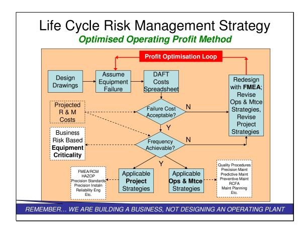
The Diagram shows a means of selecting appropriate project, maintenance and operating strategies matched to the size of risk carried by a business. The methodology is known as the 'Optimised Operating Profit Method'. It uses the more than 60 Defect And Failure True (DAFT) Costs that could happen from a failure, to determine the true cost of business risk and then matches risk control practices to the risk a company is willing to carry.
