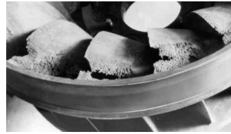
Cavitation damage on the blades at the discharge from a Francis turbine
