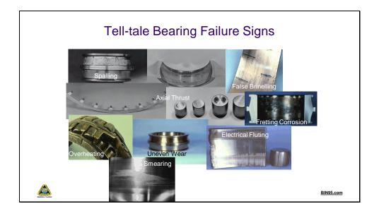
Each of these pictures of failed bearings tell the story of what caused its demise. When bearings are removed look at the 'story they tell' before throwing them into the bin. You will very likely be able to find the cause of the failure and fix it while doing the job.
