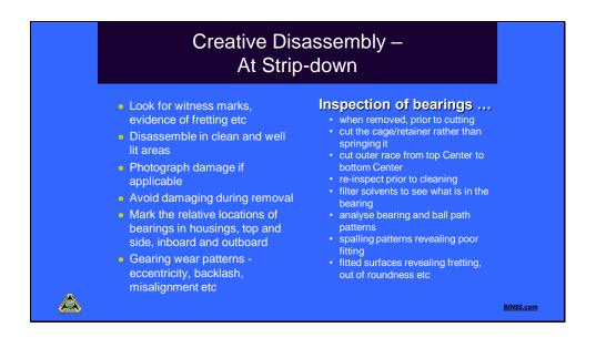
As the machine is stripped down look for evidence in its parts and assemblies for signs of what has been happening to it during use. Every part 'tells' us the story of its life; if we look for it.
