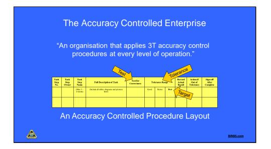
The way we write our procedures needs to change to the layout shown in the slide. This layout makes it clear to users exactly what they must achieve in every task. Each task has a boundary and test to confirm compliance. The only 'rule' is that no new task is started until the previous task is proven to be done right.
