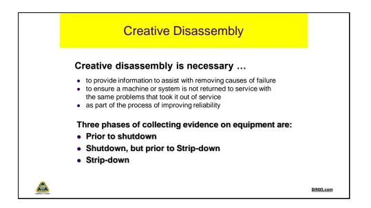
The Precision Maintenance mind set makes it necessary to remove the causes of failure as part of doing a repair. The process to adopt is known as 'Creative Disassembly'. The equipment parts provide the evidence of their demise. From the failure evidence, an analysis is conducted to identify the causes. Once the causes are known they are permanently corrected. Creative Disassembly follows a three-step process in which evidence is carefully collected to be sure the real cause(s) are found.
