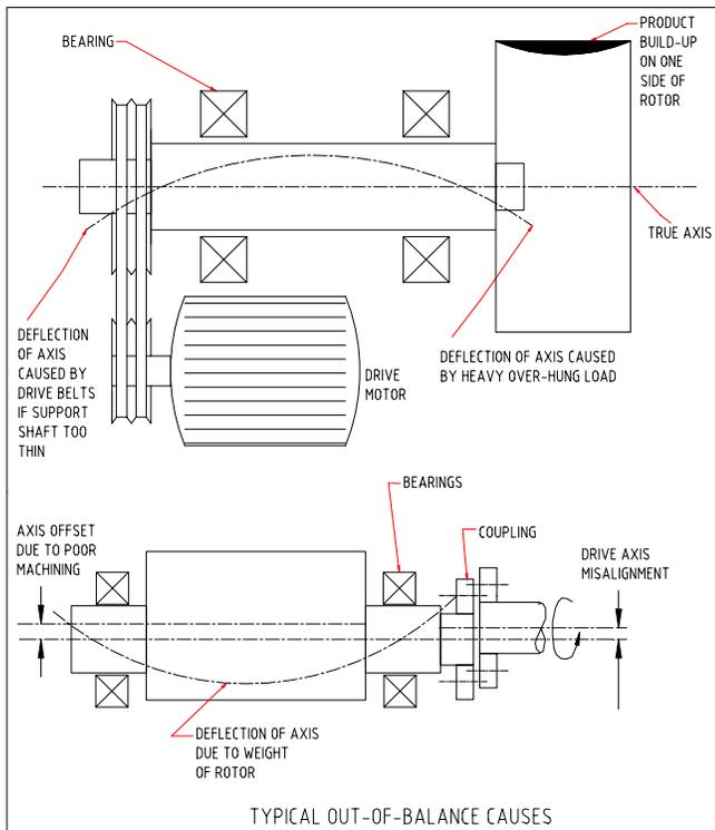
**REDUCING UNBALANCE PROBLEMS** Minimizing vibration involves minimizing out-of-balance forces. The following table indicates simple actions to take to reduce the problems of out-of-balance.
